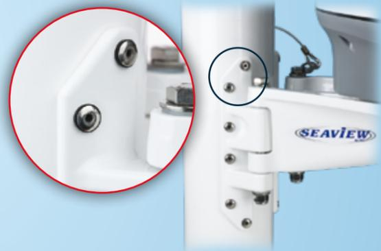
Six stainless steel rivets with nylon washers to protect powder coat finish per foot are used to hold the heavy duty mounting feet to the mast.
