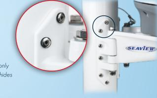
Six stainless steel rivets with nylon washers to protect powder coat finish per foot are used to hold the heavy duty mounting feet to the mast.
