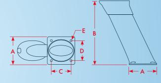
C & D E В inch / mm Model # inch / mm inch / mm inch / mm PMA-57-M1 7 / 177.8 5 / 127 5 / 127 .5 / 12.7 7 / 177.8 10 / 254 5 / 127 .5 / 12.7 PMA-107-M1 .5 / 12.7 PMA-167-M1 7 / 177.8 16 / 406.4 5 / 127 7 / 177.8 5 / 127 .5 / 12.7 PMA-247-M1 24 / 609.6 PMA-367-M1 8 / 203.2 36 / 914.4 6.5 / 165.1 .5 / 12.7
