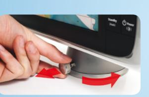
Simply pull the secure bolt out and rotate the DPOD up to 350°.
