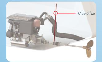
**1.** T into line after heat exchanges
