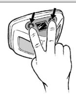
The set key can be used at any time whilst in Timer mode to resynchronise the timer to the nearest whole minute.
