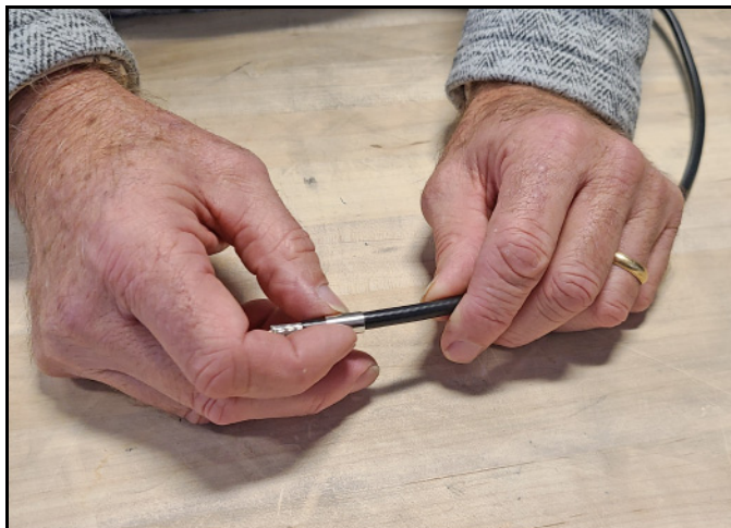
Figure 48: Placing the Ferrule
