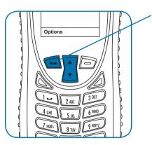
To use speaker phone: make or receive a phone call and while the call is in progress, select "Options" using the left soft key. Then, use the 2-way Navi-key to scroll down and select "Speaker" using the left soft key for "Select". To switch back to earpiece, press the left soft key again and scroll to "Ear" and press the left soft key to "Select".
