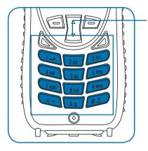
The numbered and alphabetized kevs make up the Keypad. Use the kevs to enter text, numbers and punctuation marks into various fields in display screens. See entering characters on page 61 for more information
