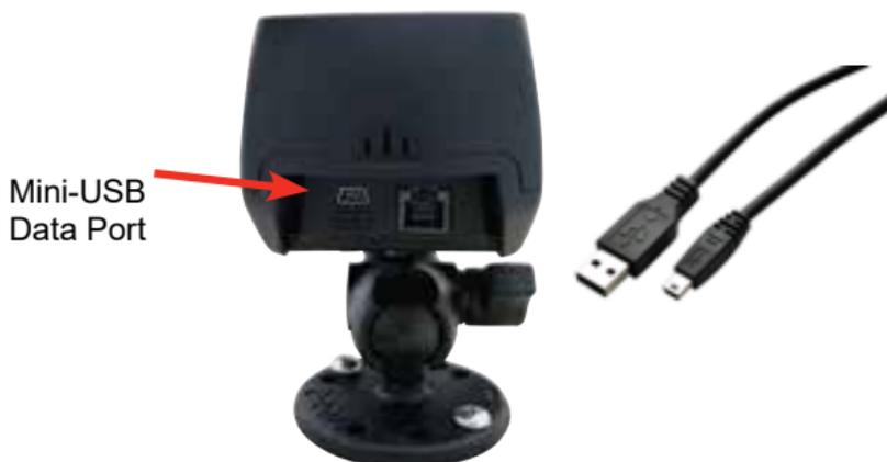
To connect a PC/laptop to the PotsDOCK bottom mini-USB port, you will require a mini-USB-B to USB-A data cable. This cable is included in your original 9555 package.
