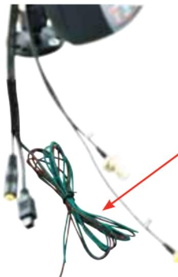
PotsDOCK provides an additional cable pair from its rear cable loom, known as the standard Beam alarm-loop. This provides a Normally-CLOSED wire loop, which can be used to connect to any passive type of button, or relay, or reed switch in which the action breaks the loop (OPEN) to activate the alarm state.
