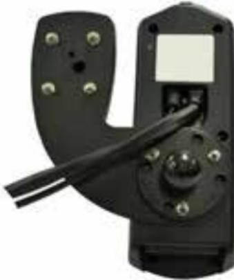
4. Plug the Privacy Handset 4-pole connector into the rear cable loom. (Please use suitable electrical tape and/or strain relief clamps where required to ensure reliable connection)
