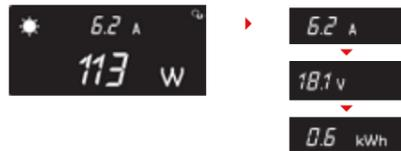
Instantaneous production power in Watt, instantaneous production current (A), instantaneous voltage (V), and production history (kWh).
