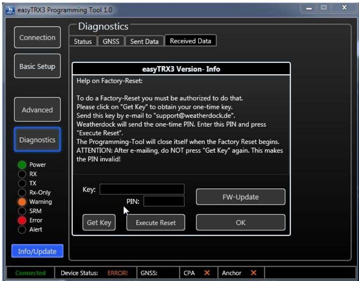
Figure: 39 Pin-code page programming tool
