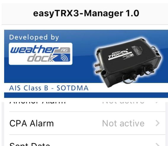
The CPA (Closest Point of Approach) alert functionality was developed to avoid collisions due to low visibility at night or bad weather conditions.
