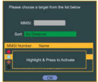
Entering any AIS MOB devices will set up the ATA100 as a Man Overboard Alarm sounding an audible warning and/or activating the build in relay to trigger a third party indicator or Alarm.
