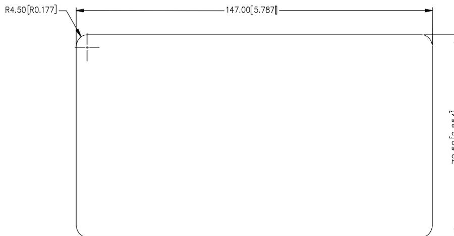
**Cut-Out & Radius Dimensions for the 1460 Control Head (NOT TO SCALE)**
