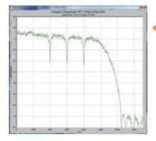
Three 20 dB notches deployed by Cygnus to maintain optimum performance.
