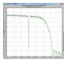
65 dB notch deployed by Cygnus to reduce in-band interference.
