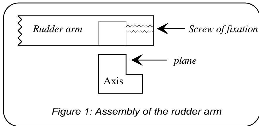
Figure 1: Assembly of the rudder arm
