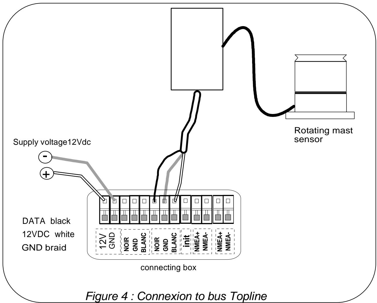
Figure 4 : Connexion to bus *Topline*
