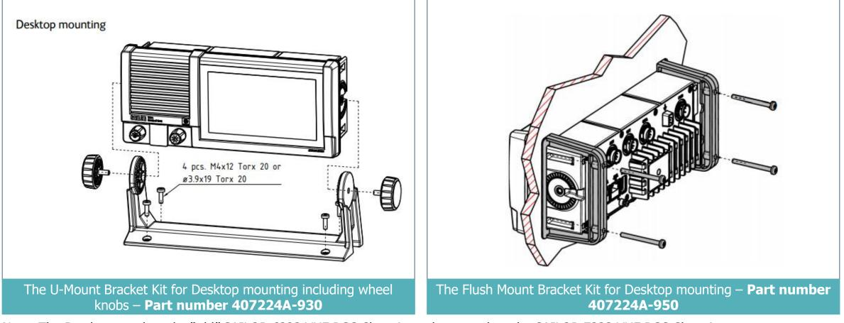
Note: The Brackets used on the "old" SAILOR 6222 VHF DSC Class A can be reused on the SAILOR 7222 VHF DSC Class A
